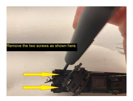
Step 3: Remove the lower portion of the rear/side handrails.
