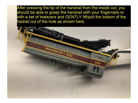
Shell can be removed now, and the decoder can be accessed:
